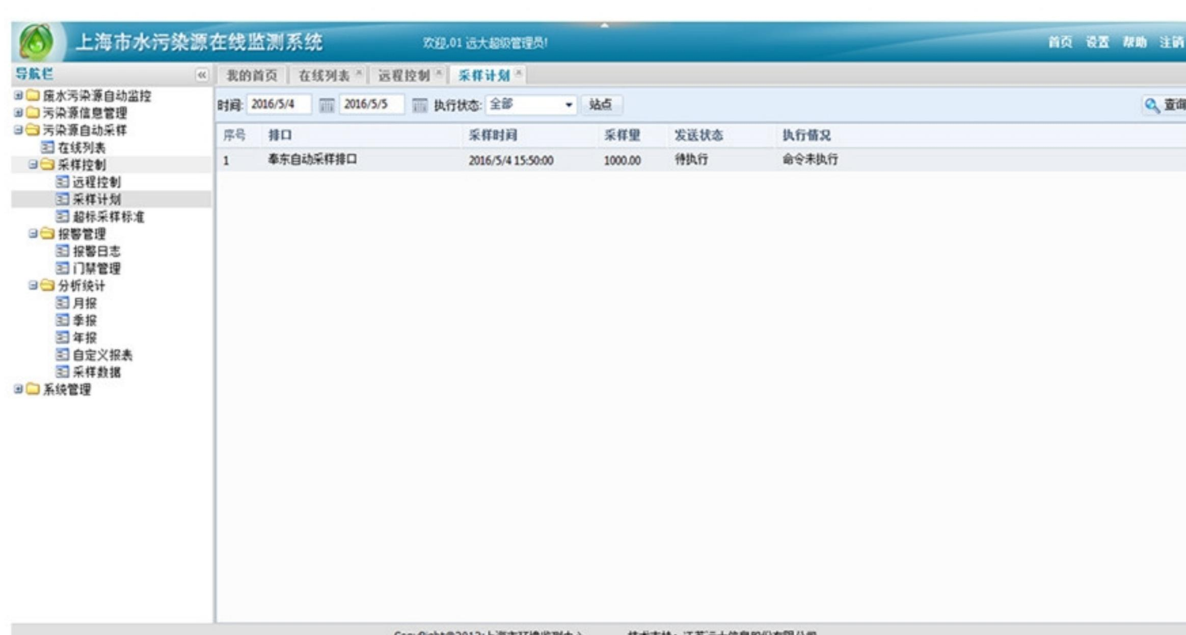
A screenshot of the 'Sampling Plan Management' section of the monitoring system. It shows a table of scheduled sampling tasks for a specific port, with columns for time, sample volume, status, and execution details.
